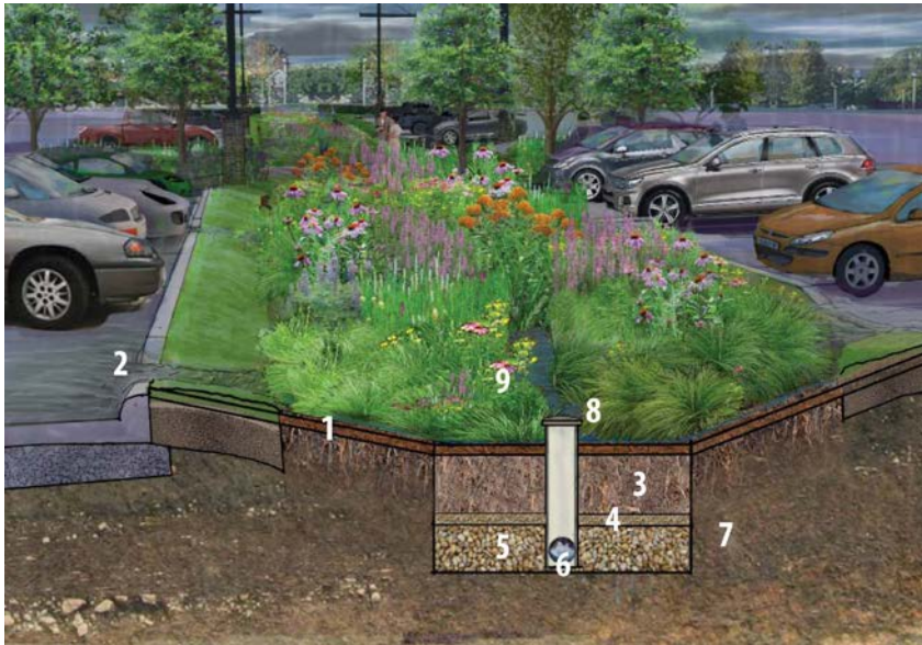
Figure 2: Bioretention cell schematic.
