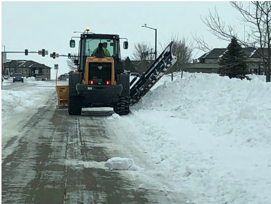
New wheel loader with blade and wing attachment
