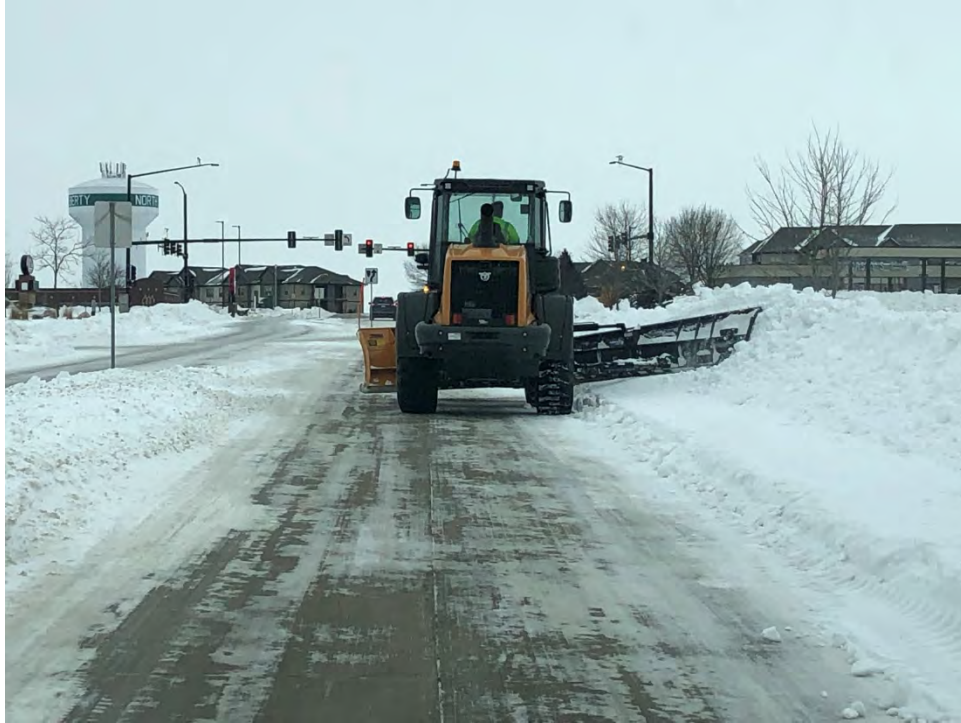
Operator pushing back drifting snow over curb. Machine was critical to keep some roads open during high wind/drifting events.
