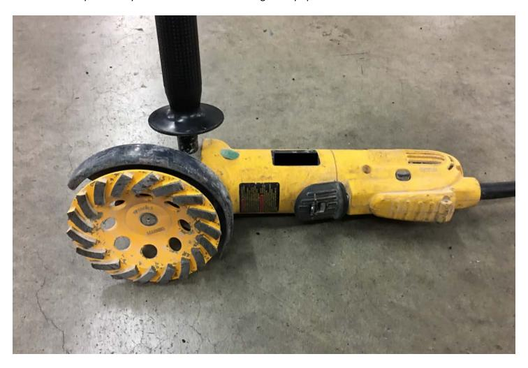
If the sidewalk is raised 1 inch or less, and the concrete edges are solid, the concrete may be ground to remove the stub toe hazard. Sidewalks raised greater than 1 inch cannot be ground, as this would compromise the structural integrity of the sidewalk.
