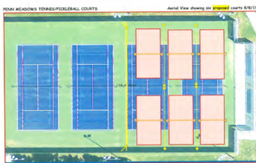
Tennis court layout replacing two of the tennis courts with the addition of 6 new pickleball courts.
