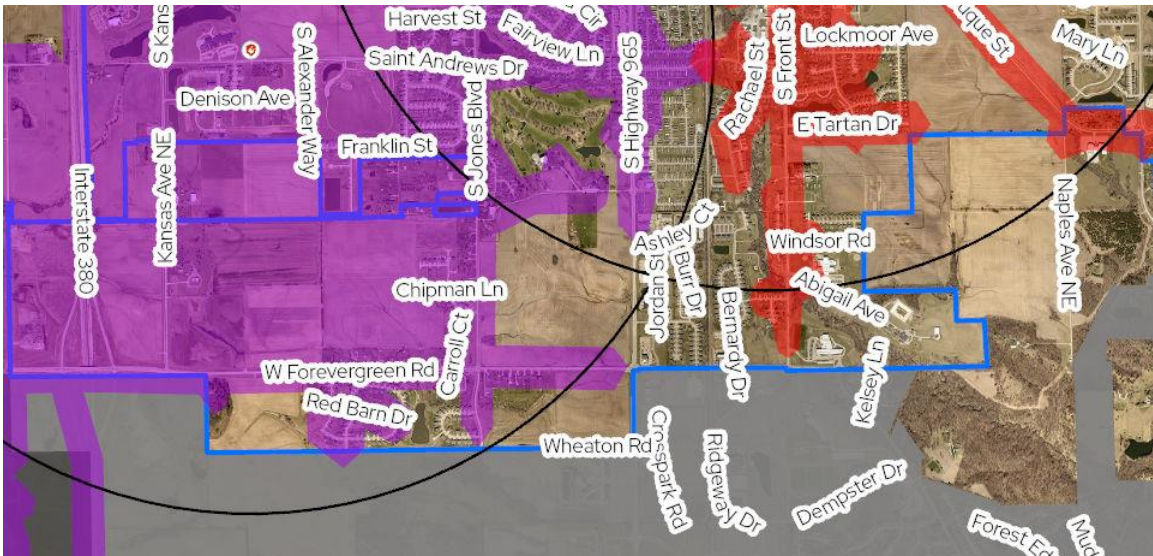
Figure 6. 1.5-mile coverage radius and 4-minute response time analysis from Fire Station No. 1 and Adjacent to the North Bend Elementary School Site.
