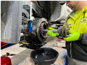
New truck axle bearing and seal replacement.
