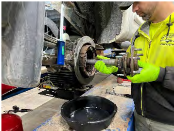
New truck axle bearing and seal replacement.
