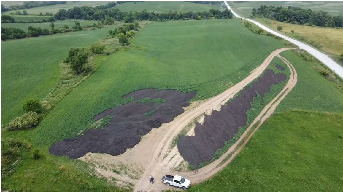
Biosolids Stockpiled at Application Site - Allows storage capacity at facility for continuous dewatering operations.
