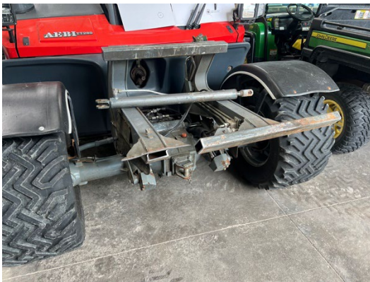
Aebi TT280 tractor front lift frame repair.
