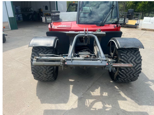
Aebi TT280 tractor front lift frame repair.
